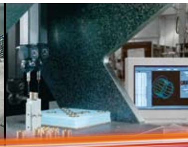
Coordinate Measuring Machines generate SPC data for quality/manufacturing consistency.
