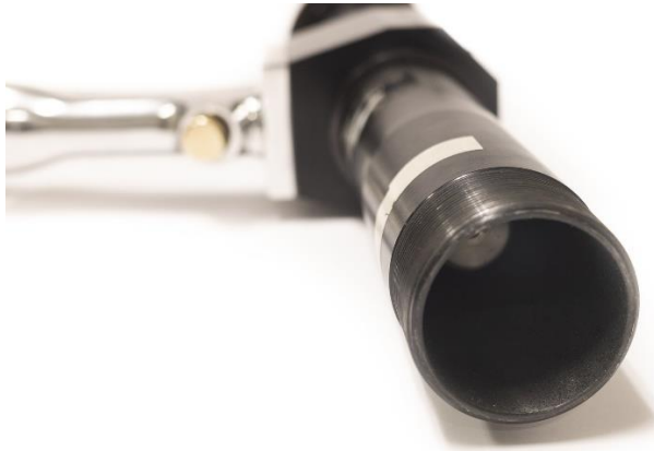
Figure 5.0-1 Medium Brute Puller Unit, Tooling Removed
