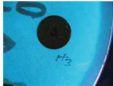
Figure 4 - Post fuel seal leak test images showing no leaks to GromEx installations.
