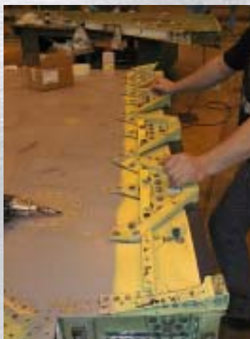
Area of interest under the wing attach fittings.
