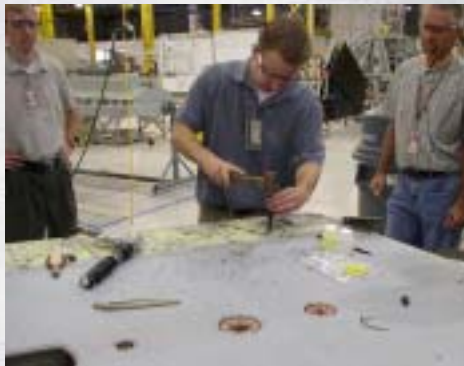
Using custom punch to remove old style nuts.
