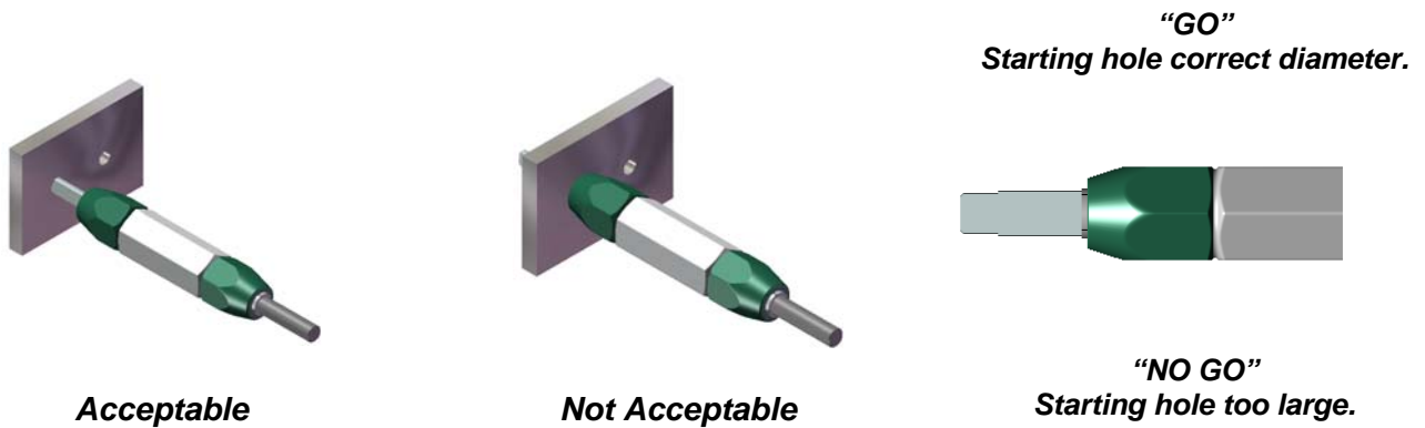
Figure 4-6 Starting Hole Gage
